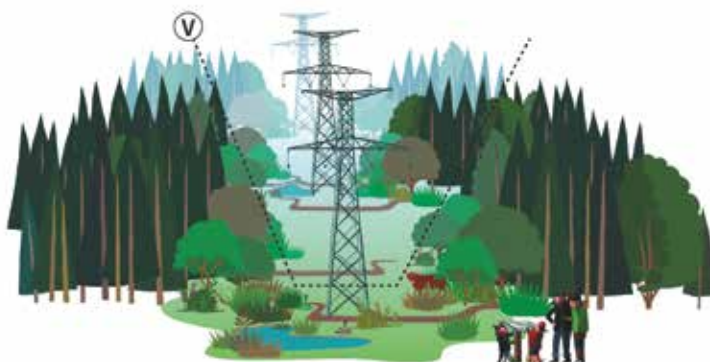
Electrical corridor in the forest in U and V shape
